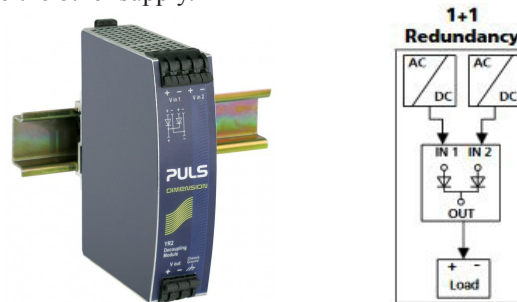
FIG. 4. Puls Dimension YR2 redundancy module. Diagram on the right depicts power flow from the supplies (top), through the YR2 diode module (middle), to the load (bottom).
