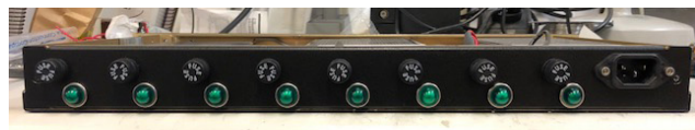
FIG. 2. Rear panel has seven circuit protection fuses and indicators, and one AC fuse with DC OK indicator.
