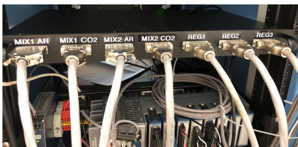
FIG. 1. Power chassis front panel has seven MFC connections.
